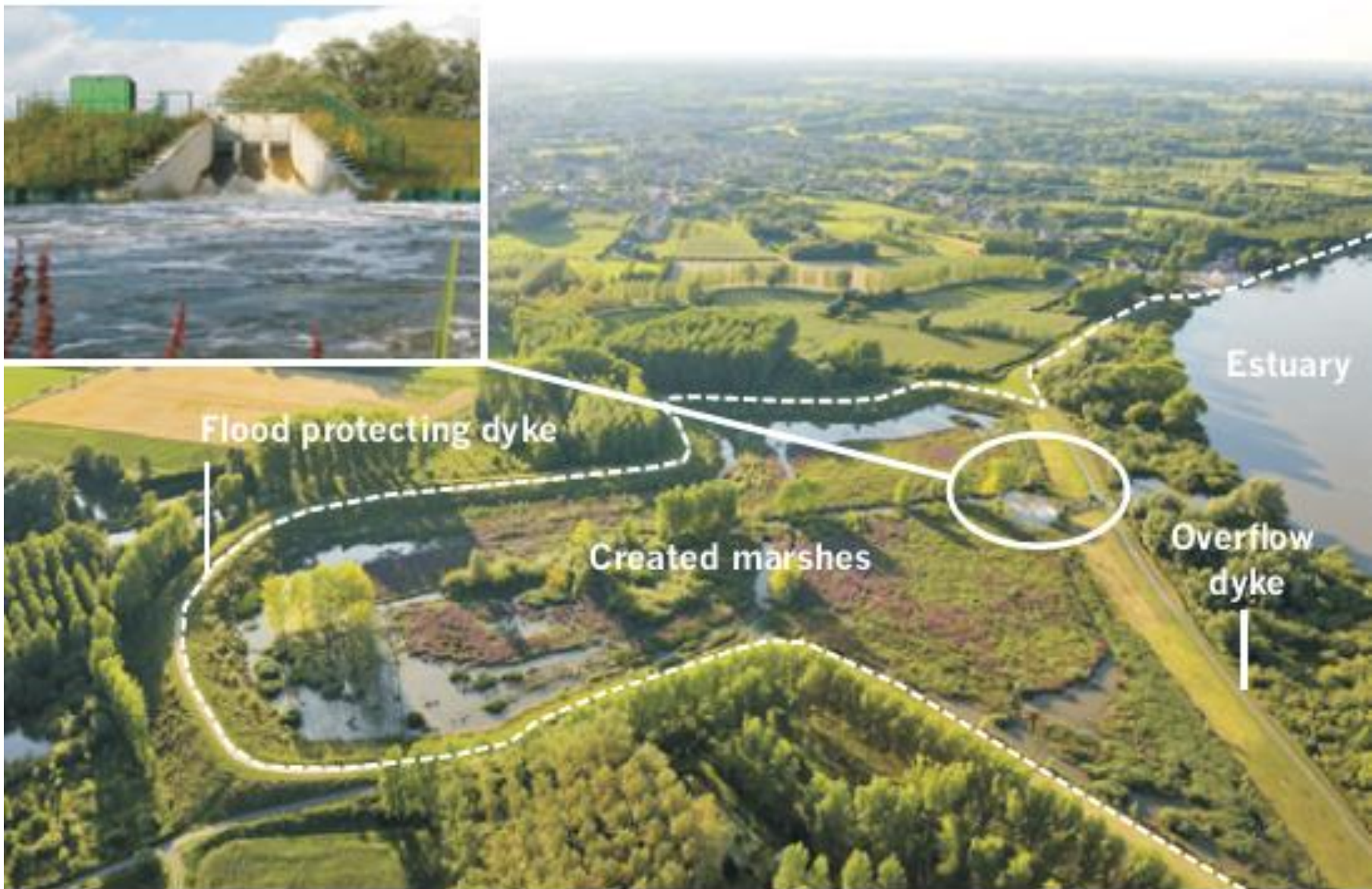
Scheldt Estuary, Belgium – protect more landward, densely populated areas from storm surges, sluice allows daily tidal flooding
